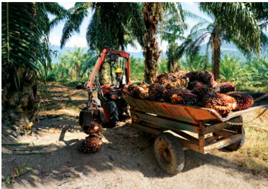
Mechanical tractor grabber for in-field FFB collection
