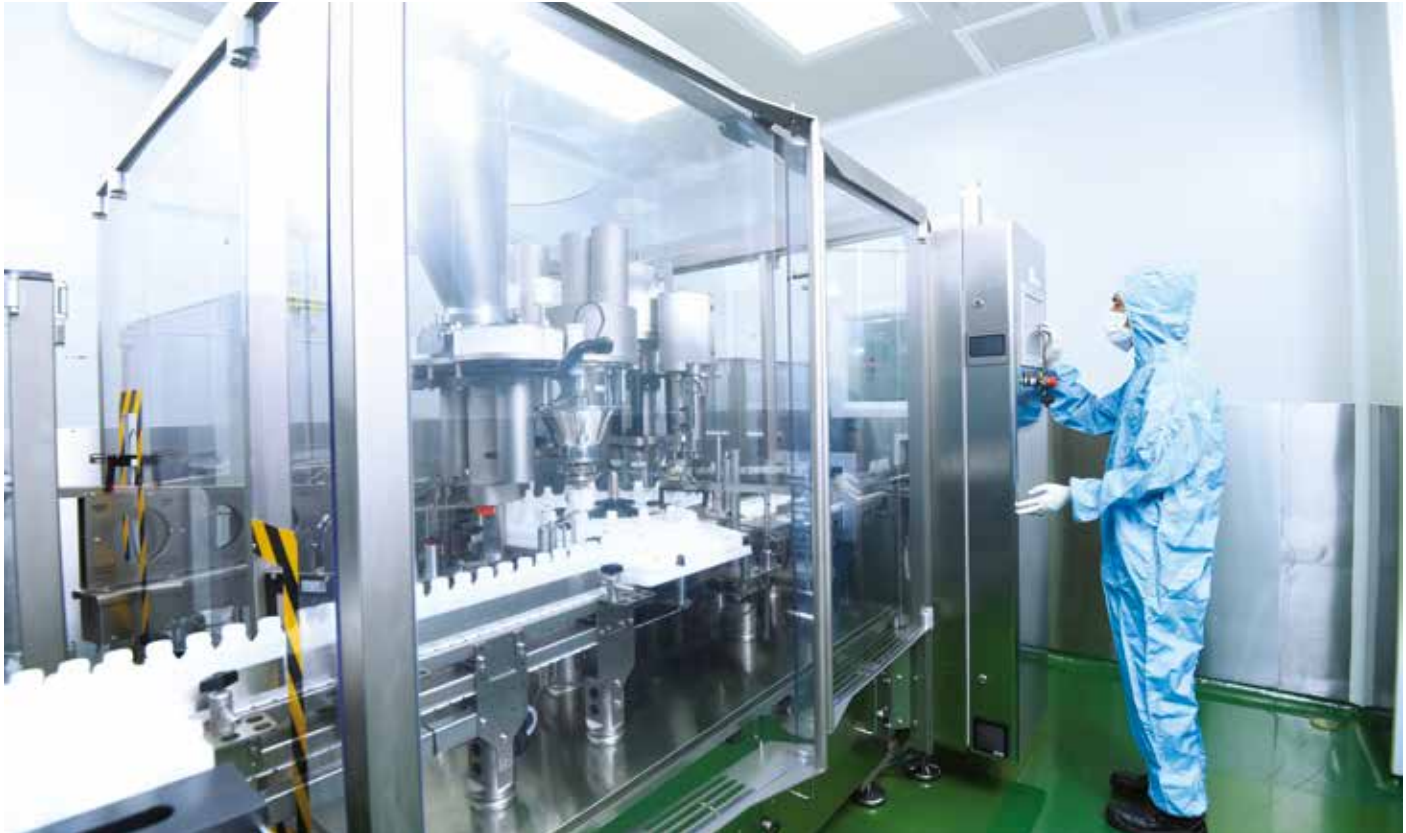
Dry syrup being filled at the filling and capping machine at our manufacturing plant in Seri Iskandar, Perak
