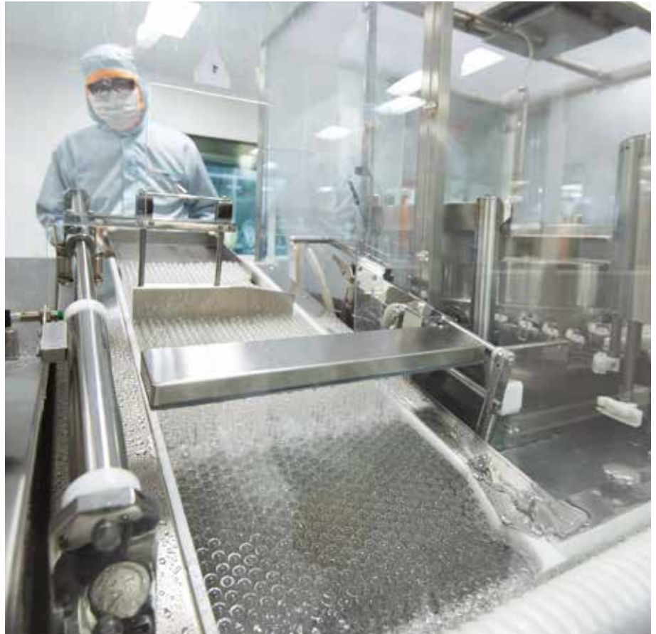
Vial washing process in preparation for Sinovac COVID-19 vaccine fill and finish manufacturing
