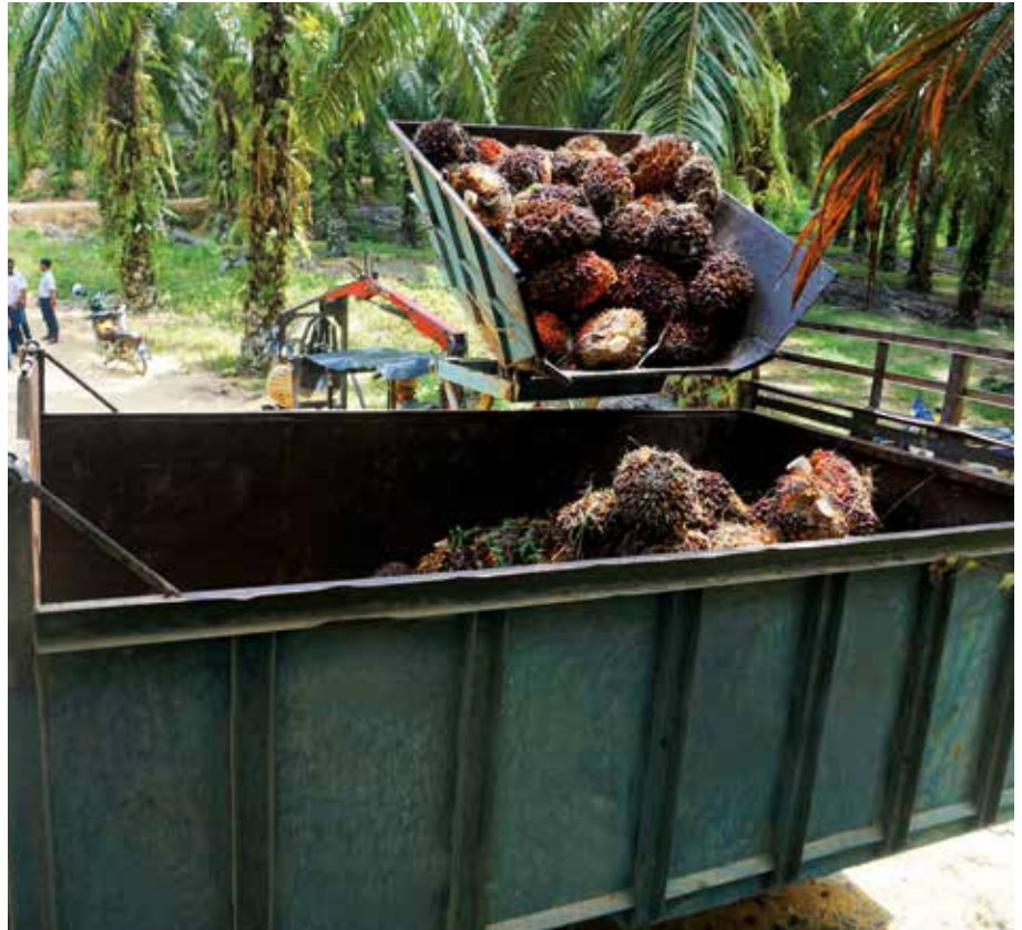
Bin system for in-field FFB evacuation
