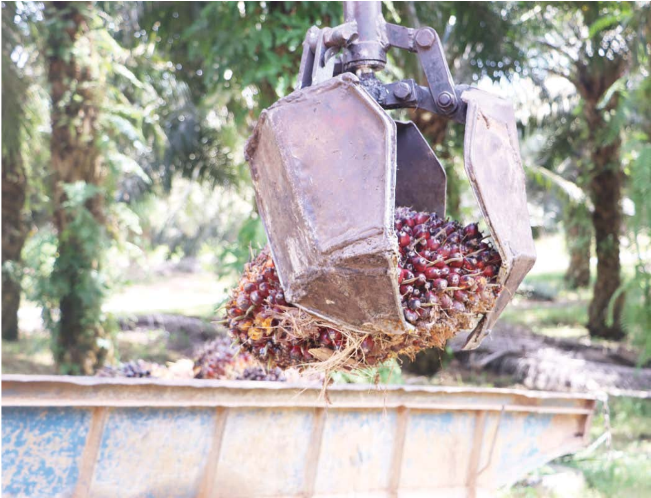
In-field fresh fruit bunch collection using mechanical tractor grabber
